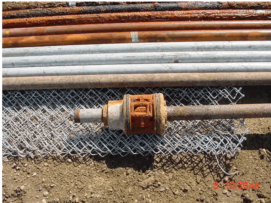
Example of New Pipe and Pipe that is Biofouled
