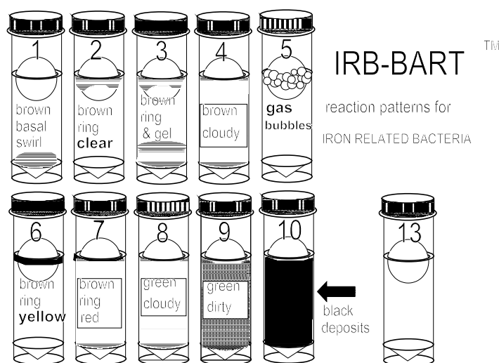
Figure 41. Eleven reaction patterns are shown above for the iron related bacteria. The presence of iron in the medium causes a variety of color reactions as well as growth forms.
